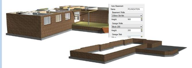
The Auto Basement command marks another leap forward for SoftPlan's powerful, time-saving automation. With a click of the mouse, you can quickly generate an automatic basement or foundation plan without the hassle of creating a new drawing. The Auto Basement feature references your main floor plan and, after selecting your walls and wall heights, creates a foundation drawing that is automatically added to the model stack.
